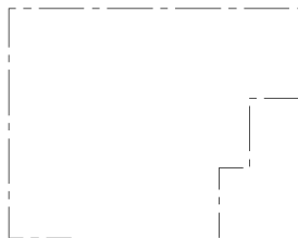
The linetype displays in a continuous pattern around the polyline vertices.
