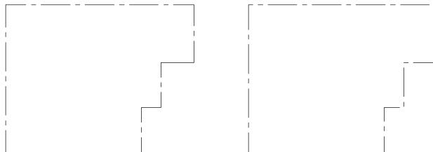
Polyline starts and ends with a dash at each vertex. The linetype will not display on parts that are too small.
