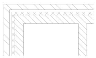
*Nota:* The result is visible in drawings generated by the BIMSECTIONUPDATE command if a multi-layered composition is attached to the sectioned solid.
