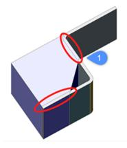
1. Collisions between a solid and sheet metal flanges.
