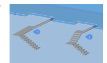
*Nota:* Press Ctrl key to cycle the possible stair types with respect to the current position of the stair cursor.
