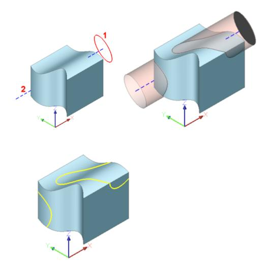
(1) 2D entity; (2) 3D solid; blue line = projection direction; pink tube = projection; yellow curves = new edges
