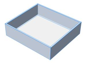
The solids are decomposed into their separate plies, which are put into one block. Each ply has inherited the BIM data of the original solid. You can see this in the Structure Browser.
