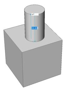
• When you highlight an entity and extrude it to the inward, a volume is subtracted from the main solid.
