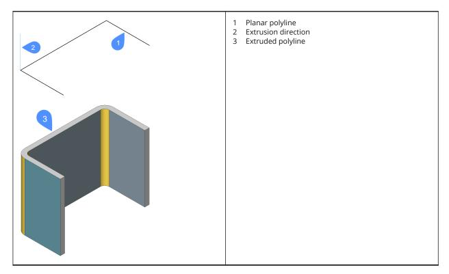
The thickening direction of the extruded surface is applied for each flange separately, to preserve the overall dimensions of polyline.
