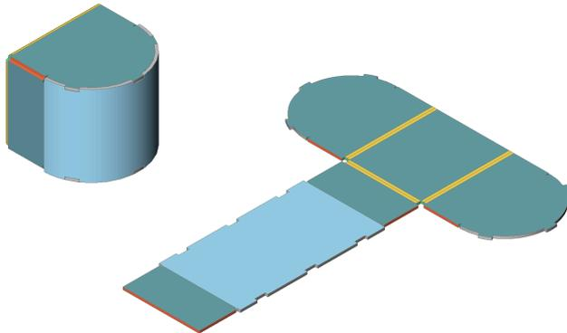
The SMUNFOLD command offers improved behavior for conical lofted bends. They can now be unfolded analytically, to avoid splitting them into a specified number of bends and flanges.
