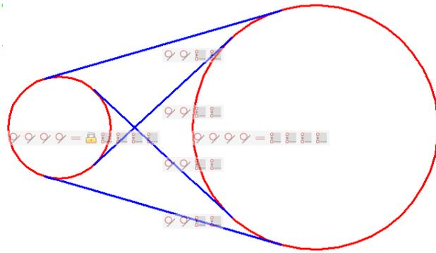
Coincident constraints between the endpoints of the tangent lines and the circles prevent the tangent lines to extend beyond the tangent points.
