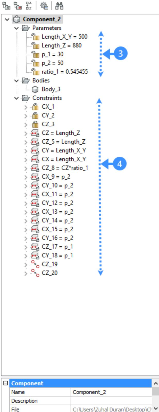
The screenshot displays the CAD Tree for a component named **Component\_2**. The tree is organized into three main folders: **Parameters**, **Bodies**, and **Constraints**.
