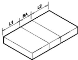
In the unfolded state of a sheet metal part, the flanges ( $L1$  and  $L2$ ) are not stretched. The bend part is indicated as BA: bend allowance. The BA equals the length of the unfolded neutral surface:
