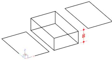
**THICKNESS** = 0 (left), **THICKNESS** = 50 (middle), **ELEVATION** = 50 (right)
