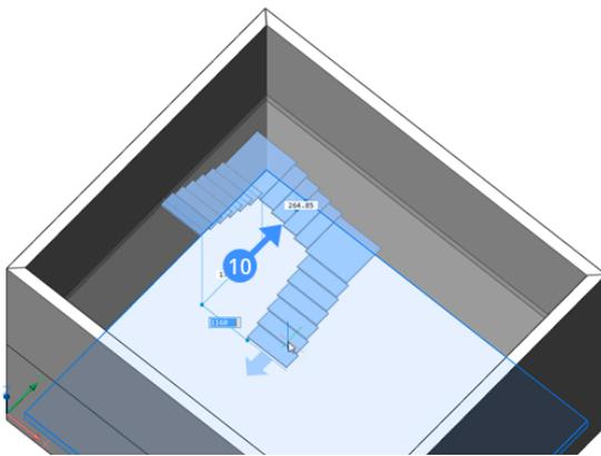
**Anmerkung:** A live preview of the flight of stairs to be created (blue) will follow the mouse dynamically (10). The **Stair** tool will automatically snap to the configurations that correspond to the current settings. When the optimal configuration is satisfied, this preview will display in a darker shade of blue.
