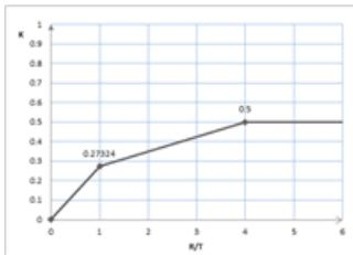
The only K-factor parameter you can control in the browser is for  $R/T$ . That means if you set the value to 0.6, the interpolation law leads to the following result:
