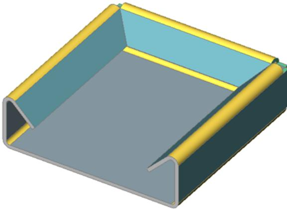
If the flanges are created externally, use the **Toggle** option (as well as **widget control**) to control the connection type for miters:
