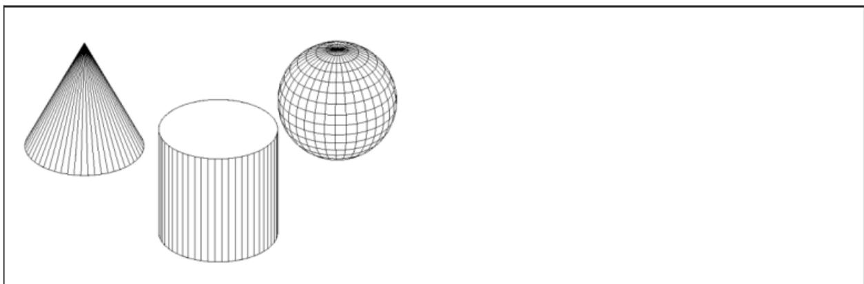
Hidden line of a cone, a cylinder and a sphere with DISPSILH Off (top) and On (bottom).
