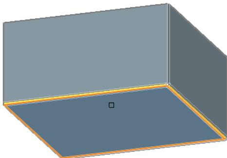
The application will compute flattening of the given part and switch it to associative mode. Condition of success of given operation is the same as for regular unfolding. Continue working in associativity mode only if no errors or warnings appeared during the operation. A new temporary document containing the flattened part will be created.
