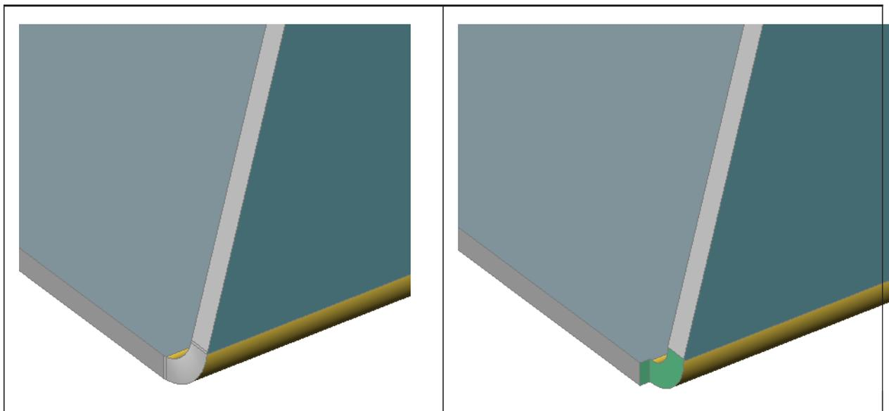
A bend relief is not needed because of a smooth transition of the geometry.
