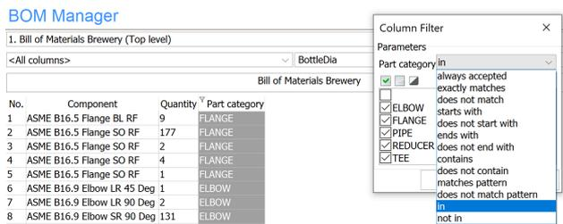
Aggregated columns are now supported in top-level and bottom-level BOM tables created with the BMBOM command. They allow you to calculate the sum, minimal, maximal or average values of a given property with respect to the current grouping.
