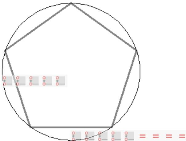
By applying coincident constraints between the pentagon vertices and the circle, and equal constraints between one side and the four other sides, the circle radius defines the size of the pentagon.
