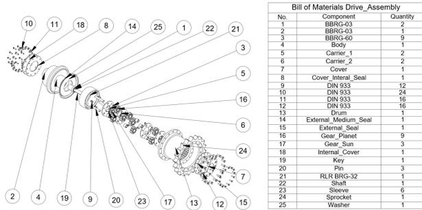
**Abbildung 30:** Example of Exploded Representation
