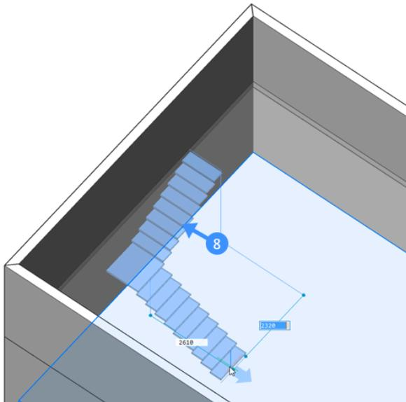
**Anmerkung:** A live preview of the flight of stairs to be created (blue) will follow the mouse dynamically (8). The **Stair** tool will automatically try to find optimal configurations of the stair that correspond with the dimensions given in the settings dialog. It will snap to the optimal configuration and display this preview in a slightly darker color.
