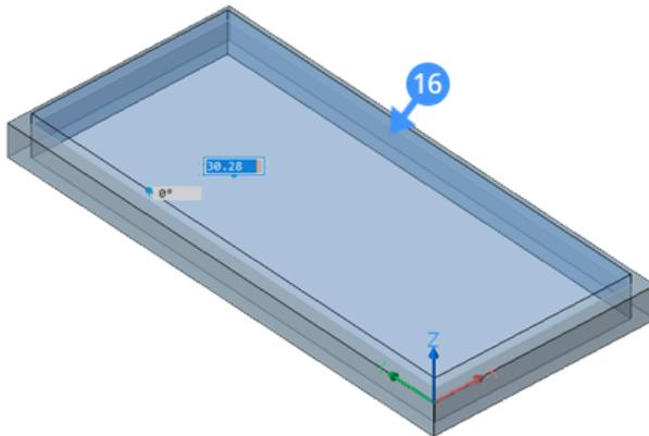
Note that to create a glass pane, the create option should be selected from the Tooltip of **DMExtrude**.
