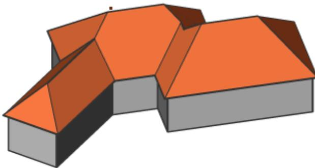
7 To define the thickness of the roof solid we will use the **Body/Shell** option of the SOLIDEDIT command.
