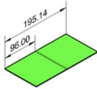
This value fits the formula exactly: a straight angle in radians roughly equals 1.57 (PI/2). The default K-factor 0.27324 gives an Unfolded Length = 196.
