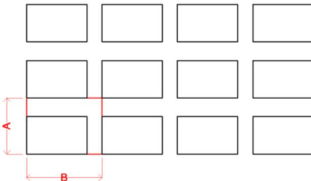
Row offset (A) and column offset (B) can be defined by the spacing rectangle (red).
