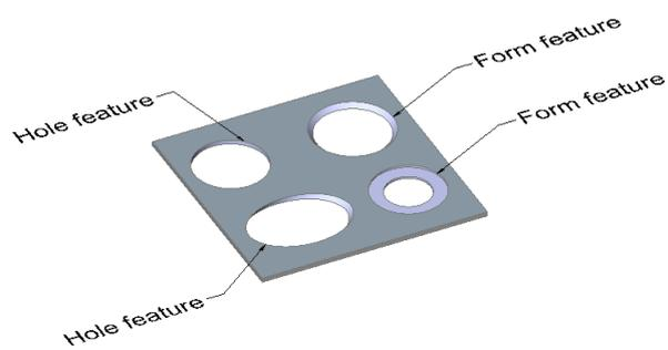
Hole features are recognized by the *SMCONVERT* command if the *SMCONVERTRECOGNIZEHOLES* user preference is ON.
