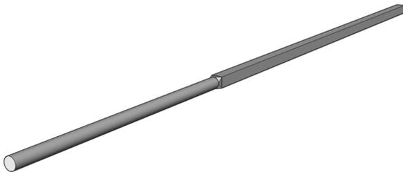
**Anmerkung:** If you had chosen to draw with a non-HVAC profile, you will not get the automatic classification as Flow Segment and the connection will not be made immediately. You can still manually classify the profiles through the BIMCLASSIFY command and then use BIMFLOWCONNECT to connect the two through a reducer.
