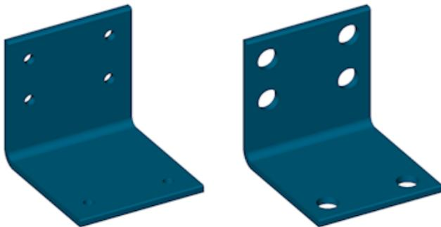
Apart from the recognition of equal radii, BricsCAD automatically recognizes other geometrical relations between surfaces of a solid and preserves them during direct modeling operations.
