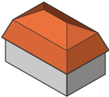
A mansard roof is composed of two solids, which we will create as two separate extrusions.
