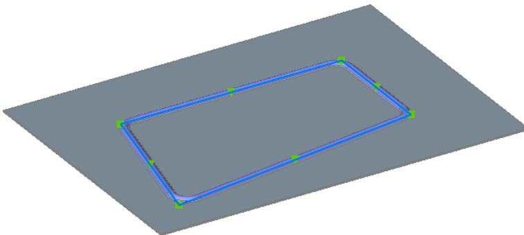
This illustrates the associativity between the 2D curve and 3D rib feature. The recognition of rib features in *SMCONVERT* is controlled by the *SmConvertRecognizeRibControlCurves* user preference.
