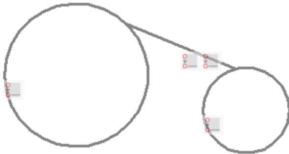
Coincident constraints between the endpoint of a line and two circles.
