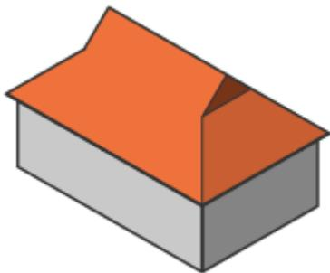
A Dutch gable roof is based on a hip roof.
