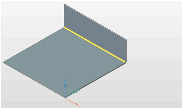
To create an edge flange where the width is different to the width of the edge, select the **Width** option of the *SMFLANGEEDGE* command and define the offset distance from one or both sides of the edge.
