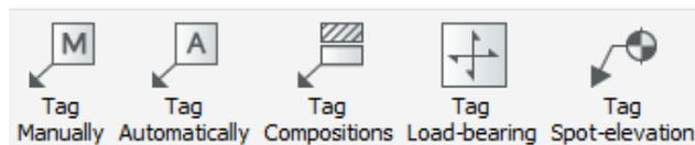
Automatically generated tags can have an offset, which is defined through the Offset attribute in TagTypeToStyle.xml found in the **SUPPORTFOLDER > Bim > Sections** folder. If the offset is not specified, the center of the tag block will be used.
