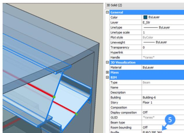
The profile data of a beam in the properties panel (5). BIMIFY recognized the profile of these model elements as structural members and detected the axis location of the profile.
