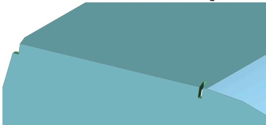
We created 2 bend reliefs because a hard edge side with a "free" vertex needs a relief in order to make orthogonal thickness face.
