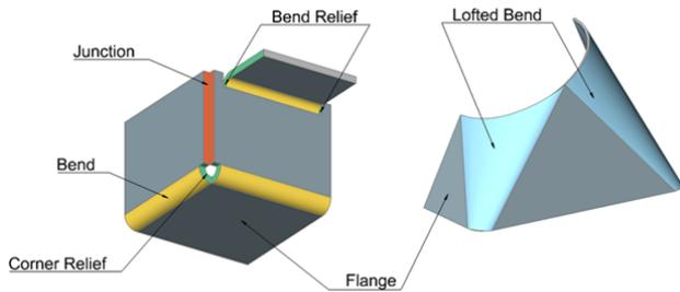
Abbildung 112: Example 1 of sheet metal features
