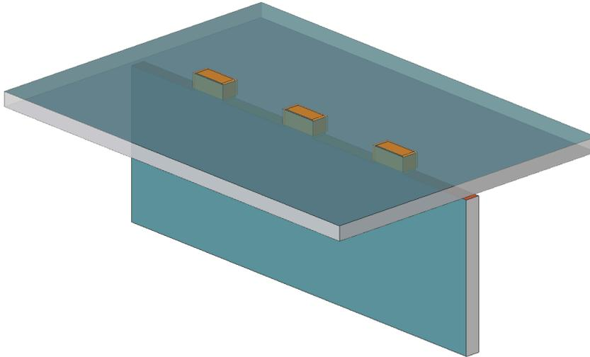
T-tabs can be created from T-junctions by the *SmTabCreate* command. T-junction features are often used as an intermediate stage for making T-tabs.
