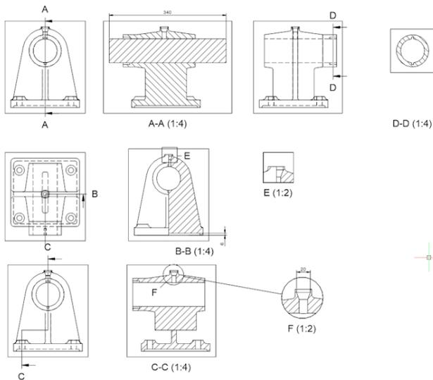
The VIEWBASE command generates associative orthographic and standard isometric views of a 3D solid model in a paper space layout.
