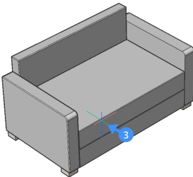
The following illustration shows inserting a Revit family sofa when both DYN and DUCS are on.
