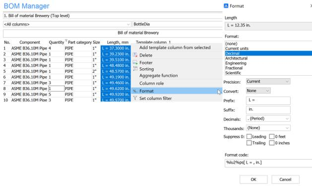
The new Column Role option allows you to specify which column should be the source of balloons for drawing views.
