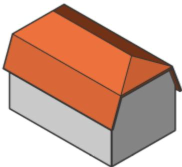
A jerkinhead roof is composed of two solids, which we will create as two separate extrusions.
