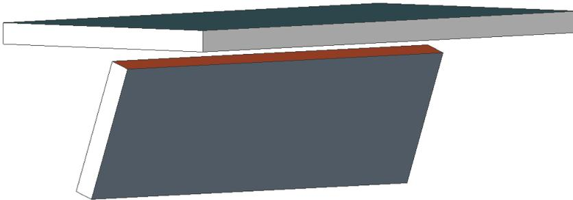
Junction features are created by *SMFLANGEEDGE*, *SMJUNCTIONCREATE* and *SMFLANGECONNECT* commands.
