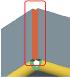
A T-junction feature consists of a thickness face of a single flange, which is located near a face of another flange,. Usually, a T-junction precedes creation of a T-tab.
