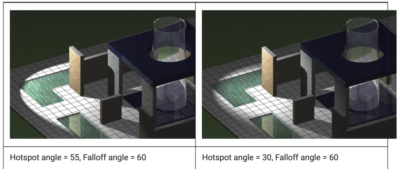
The difference between the hotspot angle and the falloff angle defines the area of lesser light intensity. If the falloff angle and the hotspot angle are almost equal the edge of light cone is rather sharp (left). The greater the difference between both angles, the softer the edge of the light cone (right).
