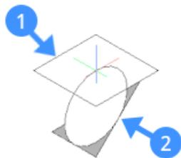
The section plane (1) lies in the XY-plane of the current coordinate system (WCS or UCS). The view direction (2) is in the negative direction of the current coordinate system.
