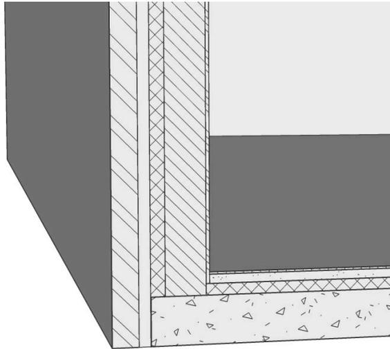
*Elevation level of interior ply is higher because ply does not reach till the base level of the floor.*
