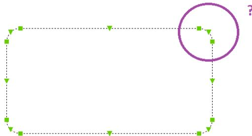
To be precise, the area of automatic junction creation is located to the common vertex of hard edges (or corner relief when bends are created). The option does not optimize the layout of the unfolded part.
