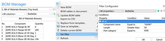
Template Columns are a new type of evaluated column, which allow you to combine values of several properties into a single BOM column, as text, using DIESEL expressions.
