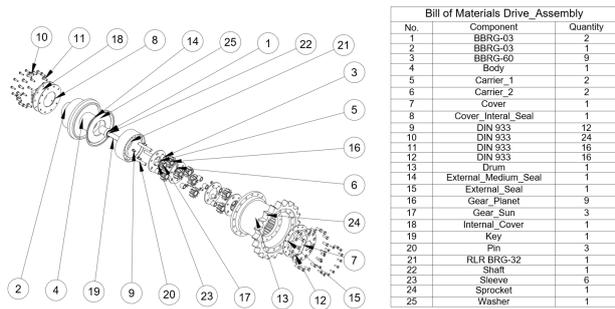
It is possible to generate drawing views for a selected exploded representation. Normally, an orthogonal projection is used for that; however, BricsCAD allows you to create any standard projection for exploded representations. Sections and detailed views are also supported.
