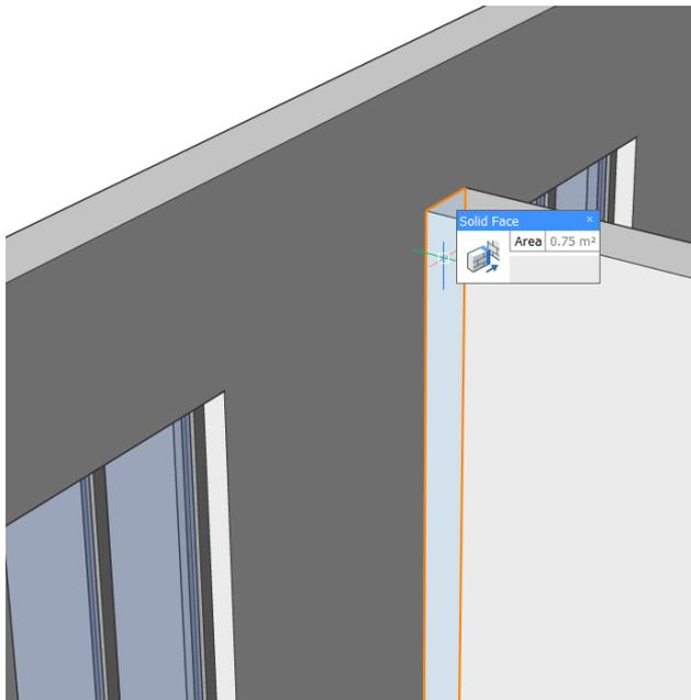
The Connect with Nearest tool automatically makes a T-connection between the two walls by extruding the face of the first wall to the face of the other wall.
