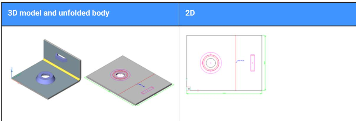
The unfold mode for the current sheet metal part can be set in **Mechanical Browser**.
