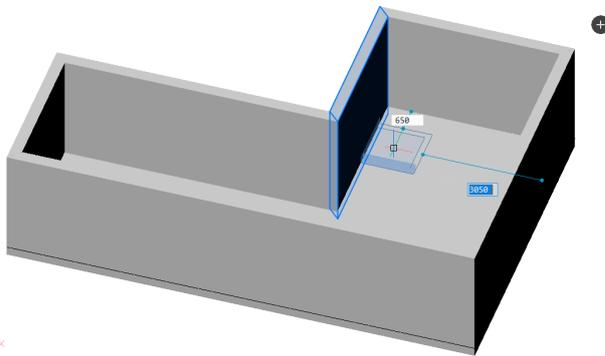
**Anmerkung:** The thickness of the wall automatically adapts to the distance between the parallel lines of the 2D drawing.
