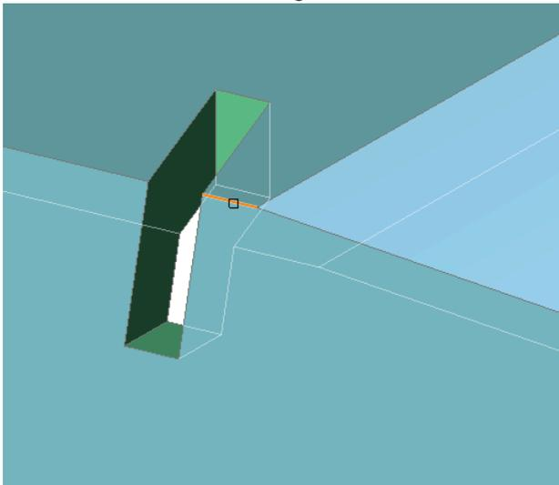
The cut is created. Parts which corresponded to linear edge get regular junction features.
