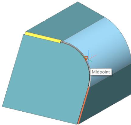
The lofted bend is split. If the connecting junction is dissolved, you can freely move the separated part.
