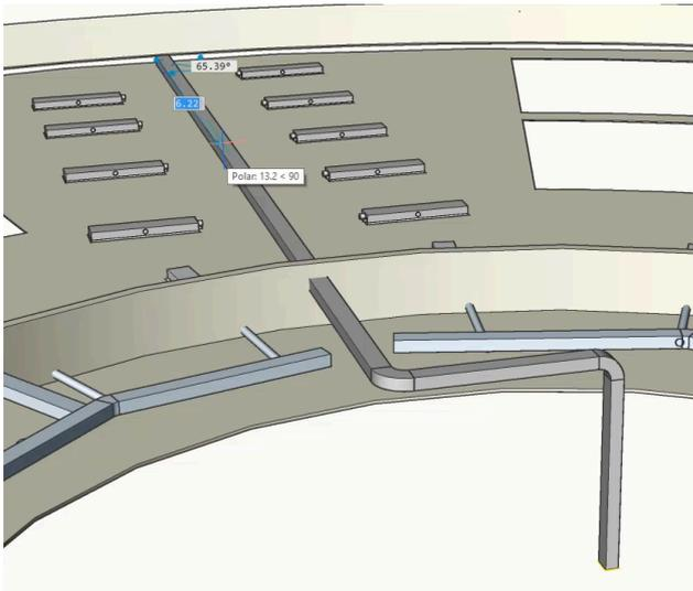
**Anmerkung:** If you had chosen to draw with a non-HVAC profile, you will not get the automatic classification as **Flow Segment**. You can manually classify the profiles through the BIMCLASSIFY command as **Building Service Elements - Flow Segments**.
