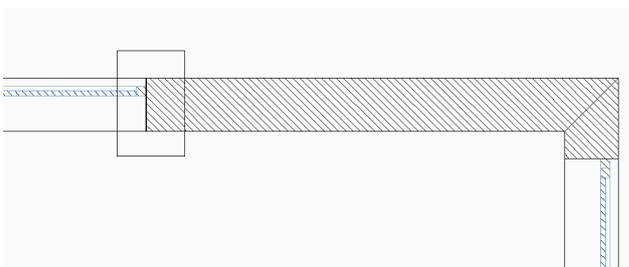
**Anmerkung:** If you would have added the vapor barrier in the model space of the section without making a patch of it, the vapor barrier wouldn't be seen as a part of the detail. If you would move your window, the vapor barrier would stay in the same position as you drew it before.
