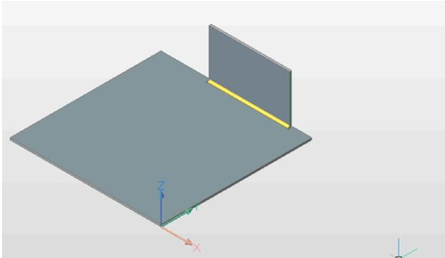
**Anmerkung:** When you create an edge flange of a different width to the edge, bend reliefs are created automatically.
