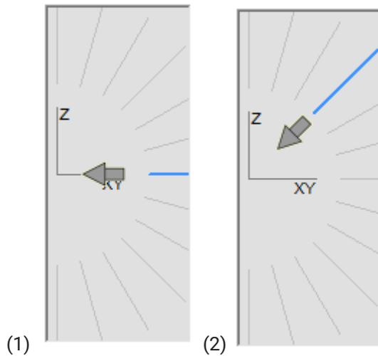
View direction is 45° down, except for 0°, 90°, 180° and 270° horizontal angles, which generate orthographic views: front, back, left and right. (3) First select the horizontal arrow, then (4) click the 45° down arrow.
