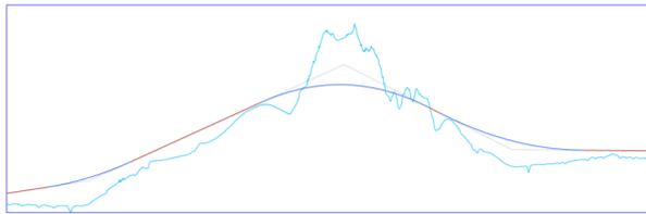
**Anmerkung:** Two vertical alignments are shown. Light blue represents terrain line from the TIN Surface, and another is design vertical alignment. The design vertical alignment has straight gradients and vertical curves and is created automatically based on the accuracy factor. You can change the accuracy factor in the Properties Panel from 1 to 100. When you choose 1 the accuracy will be the lowest.
