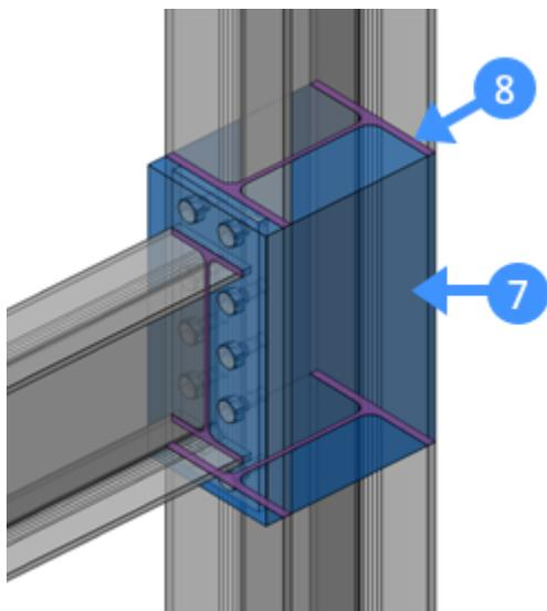
**Something interesting to note:** In this particular detail, there are holes in the column where the bolts are bolted into the column. These holes are not necessarily detail objects, but since they are part of a reference solid and they are inside the detail volume, they will be copied as well. Thus, in this respect, BIMPROPAGATE does more than a 'dumb' copy of objects.
