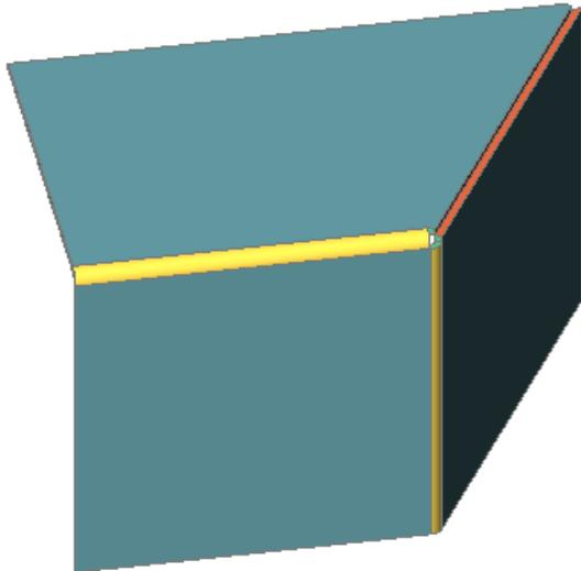
When the top bend is converted into a junction, we get to separate parts. The smart features automatically remove the now unnecessary relief.
