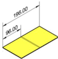
Finally, maximizing K-factor results in an Unfolded Length = 198.28. This is the maximal value one can achieve in this example since the neutral surface is taken from the external side of the bend.
