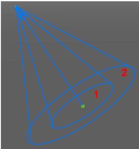
**Hotspot angle:** angle of the central light cone (defines the hotspot)
