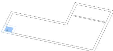
**Anmerkung:** The thickness of the wall automatically adapts to the distance between the parallel lines of the 2D drawing.
