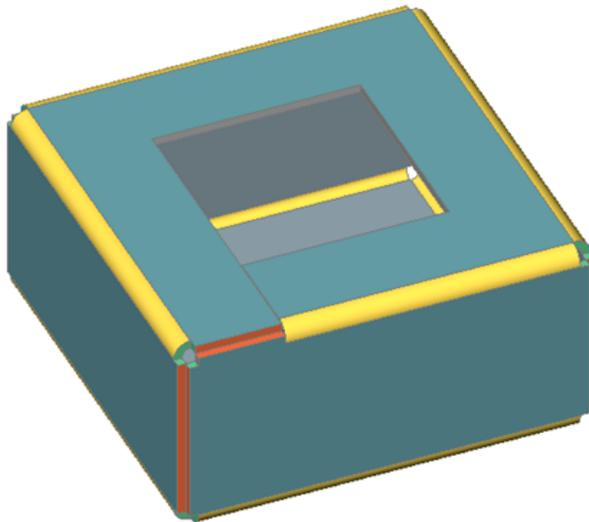
In case of the **Center** option if **Smart Features** are turned on, corner reliefs adjacent to the split will be converted into bend reliefs.
