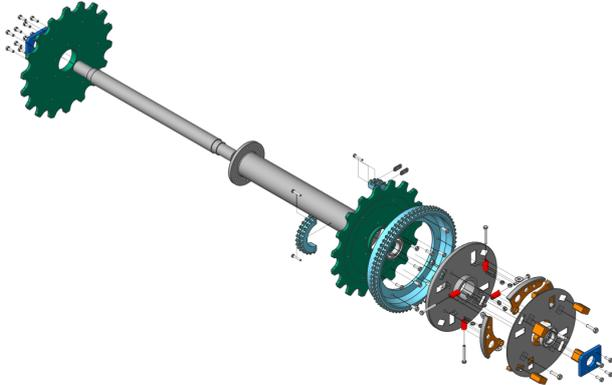
**Abbildung 32:** Example of trailing lines
