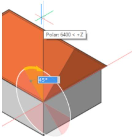
3 Execute step 7 of the Create a hip roof procedure. Remove the vertical faces of the roof solid.
