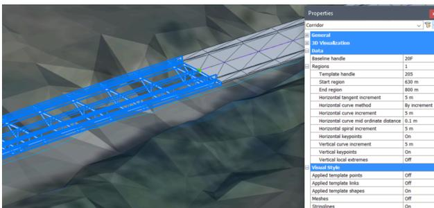
The new CORRIDOREXTRACT command enables you to extract a 3D solid, 3D mesh, or 3D polyline from a corridor to use for various purposes. For example, you can extract polylines from a corridor to use as edges for the grading. If you grip edit the alignment, the corridor and its associated geometry, such as the grading, automatically follows.
