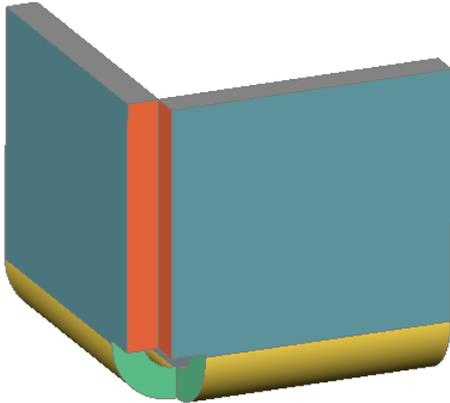
The *SMJUNCTIONSWITCH* command allows changing a symmetrical junction feature to one with overlapping faces.
