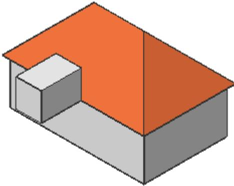
5 Select the back face of the cube: move the cursor over the cube at the location of the back face, then hit the Tab key until the face highlights (Selection Modes: Select Faces = ON).
