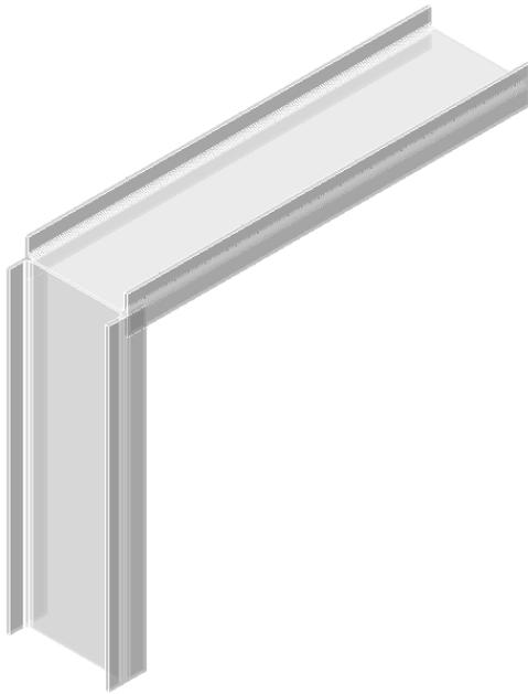
**Anmerkung:** BricsCAD doesn't automatically generate the connections between the different segments because the chosen profiles are structural steel.
