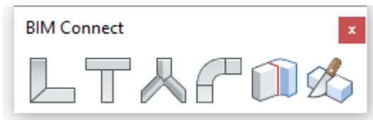
The LCONNECT command creates an L-connection (bisector or parallel) between two solids.
