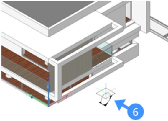
The initial section plane lies in the XY-plane ( $Z = 0$ ) of the current coordinate system (e.g. the WCS). The section plane displays dynamically and the 3D model is clipped accordingly (7).
