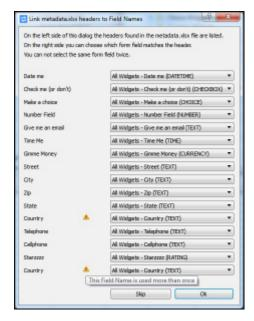
The Bricsys 24/7 Transfer Tool tries to match all field name headers provided in the **metadata.xlsx** file with the fields in the form(s) attached to the Bricsys 24/7 folder.
